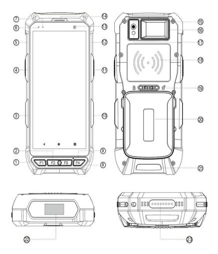
(1) F1 (2) F2 (3) Volume (4) Reserved Button (5) USB port (6) Blue Led Indicator (7) Red LED indicator (8) F3 (9) F4 (10) Power Button (11) Reserved Button (12) Reserved Pogo Pin (13) Front Camera (14) Receiver (15) Rear Camera (16) Label (17) Flashlight (18) RFID Reading Area (19) Battery Cover Locker (28) Battery Cover (20) Wrist Strap Locker (28) Barcode Scan Window (28) Cradle Pogo Pin Connector
